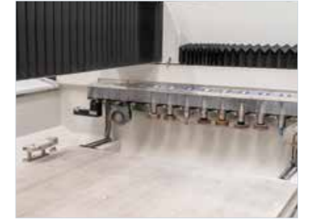
Tool magazines are located to the side for better accessibility and to offer the operator a better view of the tools in the magazine.
