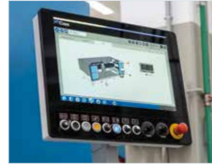
Console built into the machine, the 21.5" touch screen takes full advantage of the new operator interface. The operator is constantly guided through the most common steps while operating the machine.
