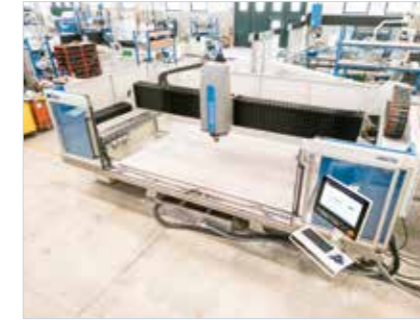
The design of the retractable doors means that the machine footprint does not change even when the doors are open.
